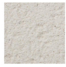
Condition 10 Render colour Ecoflend Antique White monochrome through colour smooth finish render.
