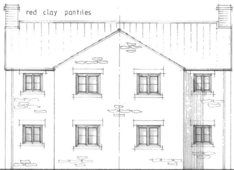
E A S T natural stone walls
