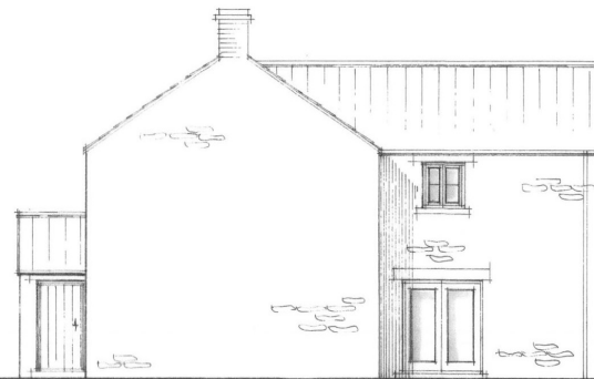
S O U T H painted timber flush casement frames in 100 deep reveals
